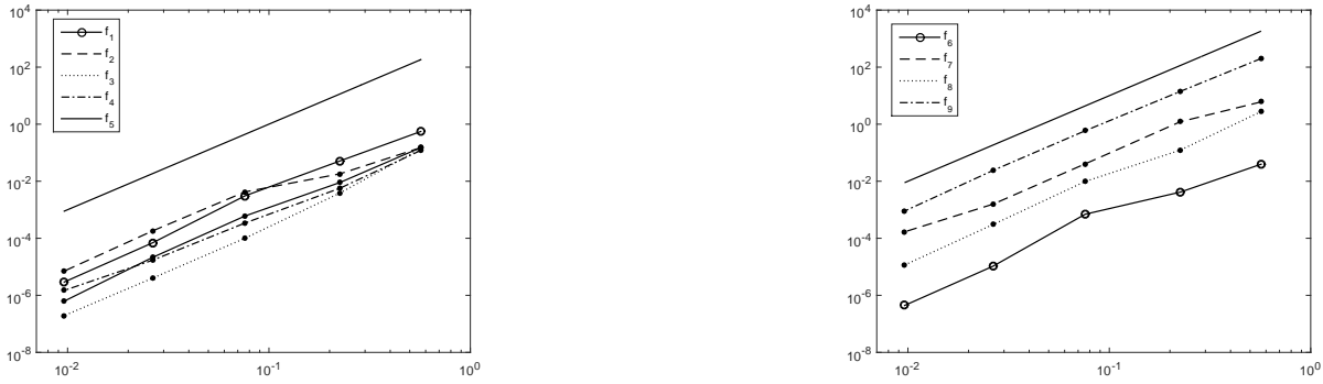
Figure 1: Log-log-plot of the approximation error of the hexagonal Shepard method. As reference, the solid line indicates a perfect cubic trend.
