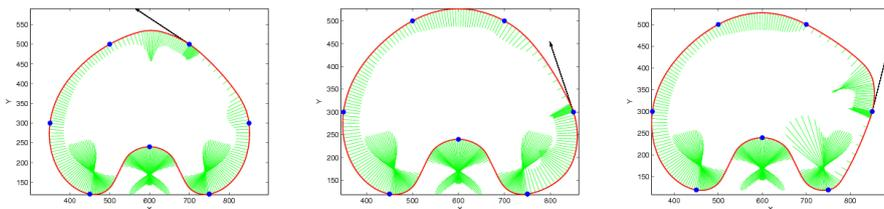
Figure 6: Interpolating given tangent vectors: the first two graphics are given tangents in different points; the last two graphics are given different tangents in the same point.
