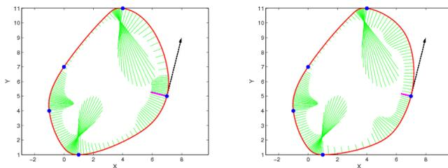
Figure 7: Interpolating same given tangent vector and different given curvatures
