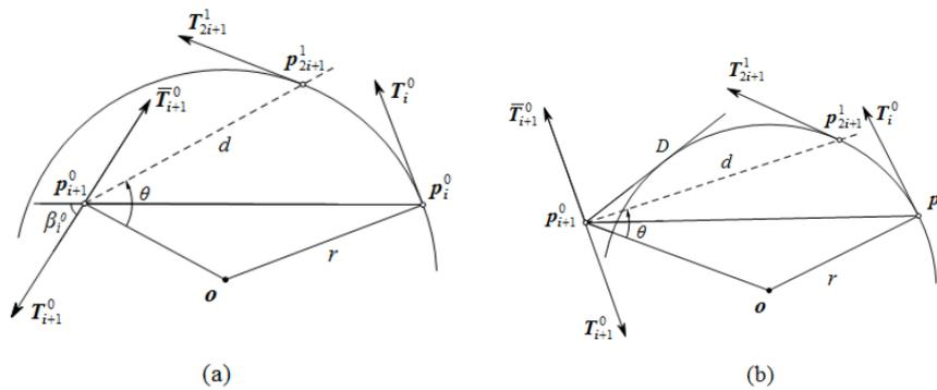
**Figure 3:** The calculation rule of new inserted point  $p_{2i+1}^1$ : (a)  $p_{2i+1}^1$  is the intersection point between the angle bisector of  $\angle \bar{T}_{i+1}^0 p_{i+1}^0 p_i^0$  and  $\odot o$ ; (b)  $p_{2i+1}^1$  is the angle bisector of  $\angle D p_{i+1}^0 p_i^0$  and  $\odot o$ .
