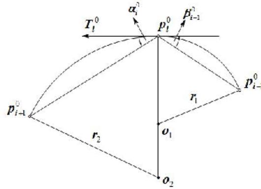
Figure 1: The definition of curvature circle at given point  $p_i^0$
