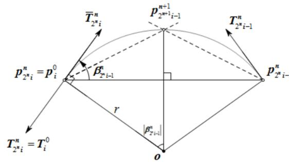
Figure 4: Analysis of Theorem 1—the limit curve interpolates given tangent vector
