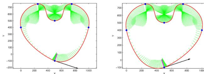
Figure 8: Interpolating different given tangent vectors and same given curvature
