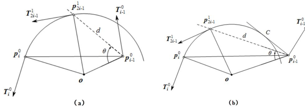
Figure 2: The calculation rule of new inserted point  $p_{2i-1}^1$ : (a)  $p_{2i-1}^1$  is the intersection point between the angle bisector of  $\angle T_{i-1}^0 p_{i-1}^0 p_i^0$  and  $\odot o$ ; (b)  $p_{2i-1}^1$  is the angle bisector of  $\angle C p_{i-1}^0 p_i^0$  and  $\odot o$ .
